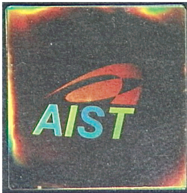
Figure 9. Color picture recorded using the laser scanning system in the thin film of the mixture of 1 and 3c (5 wt %).
